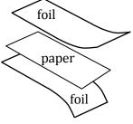
not something you need for this problem, but-adding another piece of paper and rolling the assembly will effect the miniaturization as well as doubling the capacitance as charge will now be able to be stored on *both* sides of each foil strip—clever, eh?)
